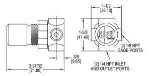
The Series MPR Miniature Pressure Regulator is a compact unit that provides low cost, high performance pressure regulation of compressed air or air/water. The low torque, non-rising adjustment knob with locking capability provides easy and precise adjustment. Models for use with air are self relieving. Models for air/water are nonrelieving.
